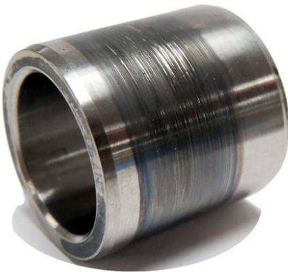
Standard Age-Hardened (STA) Ti64 Sleeve Condition after testing 1 8K Cycles, .0122"/300 Microns Wear (Stopped)
